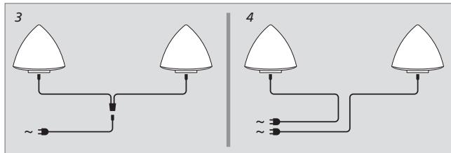
**Mains connections:** Depending on the type of mains supply connector enclosed with your loudspeakers, connect each loudspeaker to the mains as shown in either fig. 3 or fig. 4.
