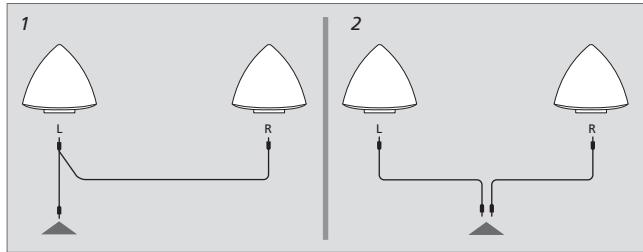
If you connect the loudspeakers to, for example, a non-Bang & Olusen audio or video system with separate connections for the left and right sound channels, make the connections as shown in fig. 2.
