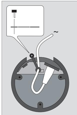
**Cable Clamp:** For safety reasons, the mains lead to each loudspeaker must be secured with the cable clamp provided.
