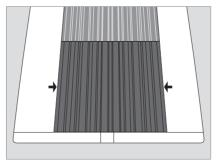
Cover for the connection panel: To remove the cover, grip it along the left and right edges – as indicated by the two arrows.
