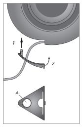
**Cover for socket panel**: *Run the two cables through the hole (A), before you connect them to the loudspeaker.*
