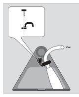
Cable Clamp: For safety reasons, the mains lead must be secured to the loudspeaker. Use the enclosed small cable clamp and screw.
