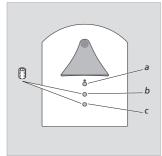
The mounting holes (b and c) are blocked by two small screws, and before you can use either of these holes, the screw must be removed.
