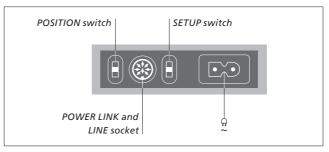
The socket panel is located on the bottom part of the loudspeaker.
