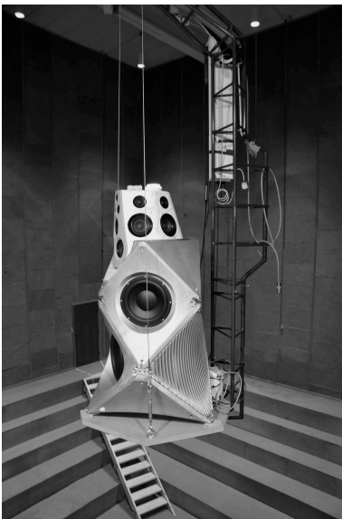
Figure 7.1: The first BeoLab 90 prototype undergoing acoustical measurements in The Cube.
