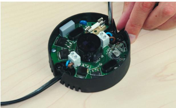
*When the wires have been connected, they are to be secured using the two black retention brackets.*
