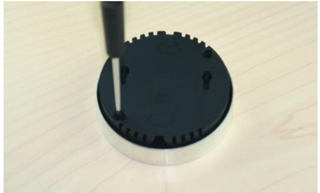
*To gain access to the screw terminals and the fuse, remove the two screws at the bottom. Now the top of the BossDim can be lifted off and the screw terminals and the fuse are easily accessible.*
