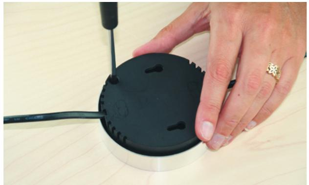
*When correctly in position the cover is secured with the two screws at the bottom.*
