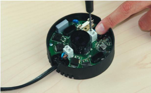
*The mains cable from the supply (mains plug) is connected to the screw terminal close to the fuse holder. The cable supplying the lamp load is connected to the screw terminals at the opposite side.*
