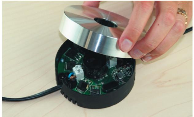
*After the wires have been correctly connected and secured, the cover is once again put in place.*
