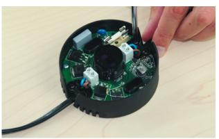
When the wires have been connected, they are to be secured using the two black retention brackets.
