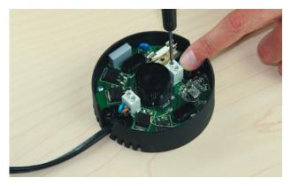
The mains cable from the supply (mains plug) is connected to the screw terminal close to the fuse holder. The cable supplying the lamp load is connected to the screw terminals at the opposite side.
